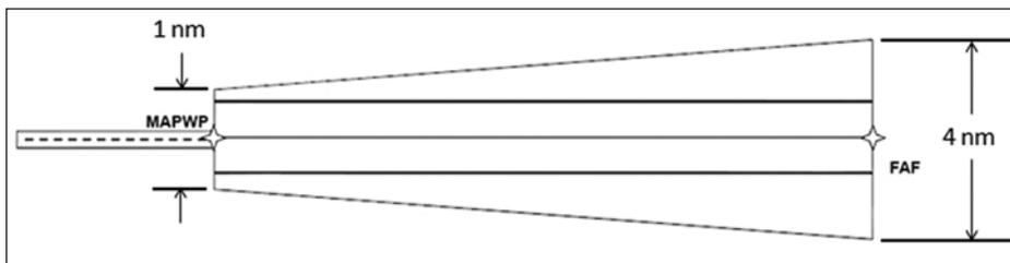
*LNAV and LNAV+V approaches use linear course guidance. The obstacle clearance area narrows from 4 nm at the FAF to 2 nm at the MAP. It is the same size for LNAV, LNAV+V and LNAV/VNAV approaches.*
