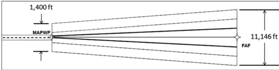
WAAS approaches use angular course guidance. LPV precision approaches allow a much narrower obstacle clearance area, narrowing from 11,146 feet at the FAF to only 1,400 feet at the MAP
